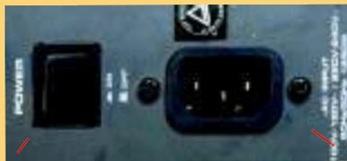
On/Off Switch    Power Supply - connect to outlet
